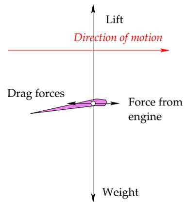
Figure 1.1. The forces on a steadily-flying plane. This figure shows the wing of the plane.
