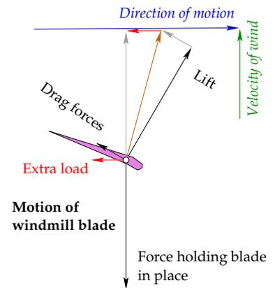
Figure 1.8. Top view of a wind turbine's blade.
