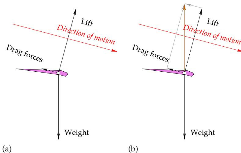
Figure 1.3. The forces on a glider, gliding steadily downhill. The lift and drag forces in panel (a) are obtained by rotating the wing and the direction of travel from figure 1.2 by a small angle. Panel (b) shows the sum of the lift and drag forces, which now points in the opposite direction to the weight.
