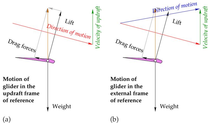
Figure 1.5. A glider, gliding steadily in an updraft. The red arrow shows the velocity of the glider relative to the air in the updraft. The blue arrow shows the velocity relative to an external onlooker.
