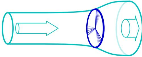
Figure 1.13. Flow of air past a windmill. The air is slowed down and splayed out by the windmill.
