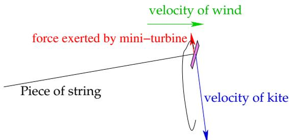
Figure 1.12. Method 1: Side view of a kite extracting power by twizzling in a circle, and generating power with an on-board mini-turbine.
