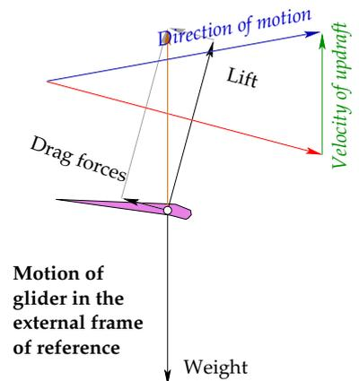
Figure 1.9. A recap of the glider in the updraft, from figure 1.5b.
