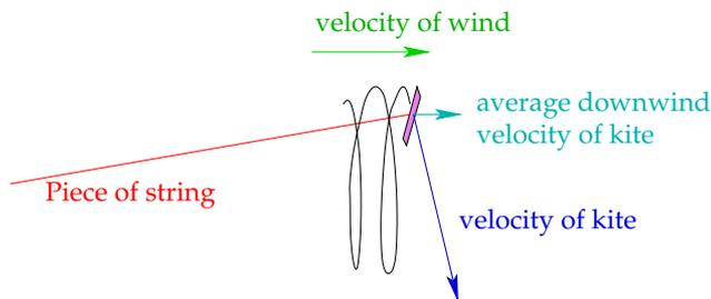
Figure 1.11. Method 2: Side view of a kite extracting power by pulling on a string while twizzling gradually downwind.
