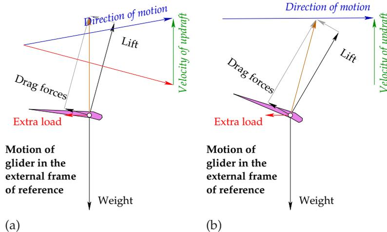
Figure 1.6. Getting work from the glider in an updraft by adding a horizontal force. (a) Force added. (b) Wing and direction of travel rotated so as to keep steady flight.
